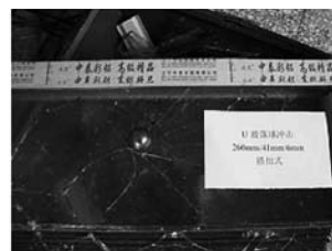
6mm U玻构件227g球1.8米冲击
